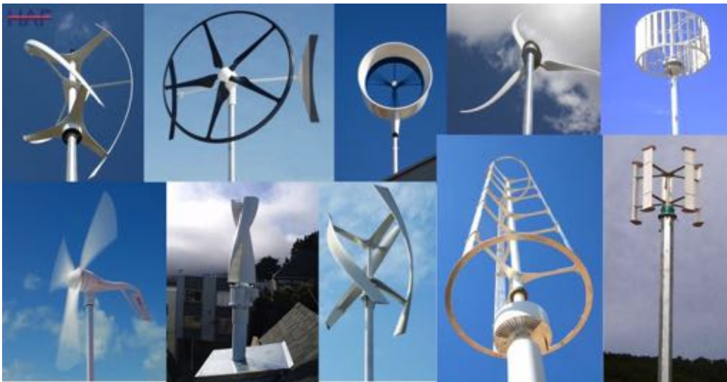
Figure. 9.2: Several micro wind turbine designs. From S.Arora by permission
