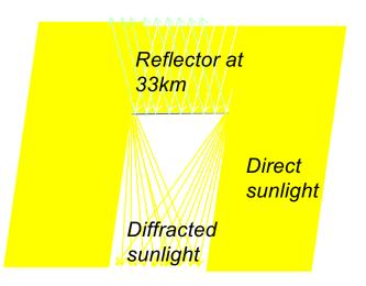
Reflectors would not be visible from the ground 100,00 feet below, day or night. Underside is black, like outer Space, to absorb radiant heat from the surface at night and radiate out into Space.
